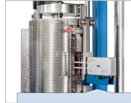
High temperature furnaces up to 1600 ° C.
