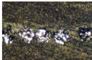
Boron-graphite composite sectioned with medium grit diamond wafering blade. Boron fibers damaged.
